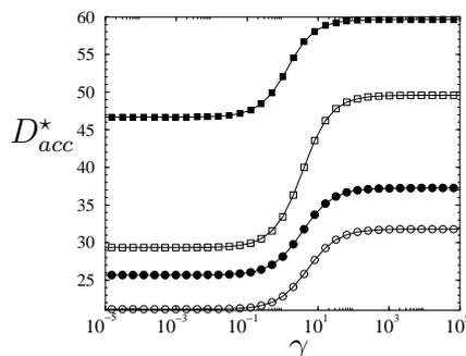
Figure 1: Computation of the accessibility domain  $D_{acc}^*$  for a Robin boundary condition versus the parameter  $\gamma$  and for  $N = 0$ . The four weighting functions  $w$  considered on table 3 have been analysed. Circular black symbols stands for the flow-averaging method with  $w = v/\langle v \rangle$ , and circular white symbols for the classical uniform volume averaging  $w = 1$ . White square symbols are for  $w = 1/(2r)$  and black square symbols are for  $w = 10(1 - r)^3$ .
