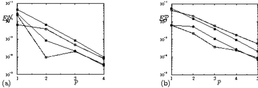
Figure 4: Same conventions as figure 2 for the relative error for non axis-symmetrical  $N = 1$  eigenvalues  $l_{1,0}$  (a) Relative error  $E_0^N = |\lambda_{0,p}^N - l_{1,0}^N|/l_{1,0}^N$  between the predicted eigenvalue and the theoretical Neumann one  $l_{1,0}^N = -4.160532810$ , versus the order  $p$  of the approximation. (b) same conventions for the first Dirichlet eigenvalue convergence  $l_{1,0}^D = -10.69115115$  with  $E_0^D = |\lambda_{1,p}^D - l_{1,0}^D|/l_{1,0}^D$ .
